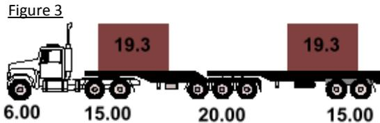
Notice that the prime mover axle loads in figure 3 are less than those in figure 2.
