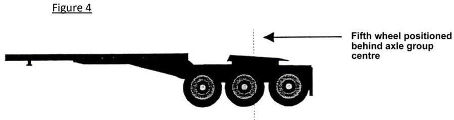
It is also important to understand the effects that the positioning of the load on each trailer will have on the individual axle loads.
