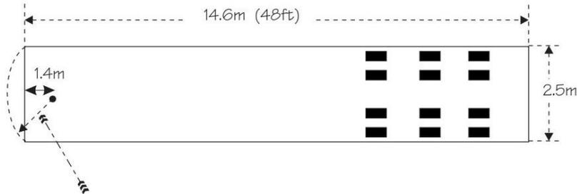
The forward projection must be contained within a 1.9 metre radius from the king pin, which equates to 1.4 metres to the front of the trailer.
